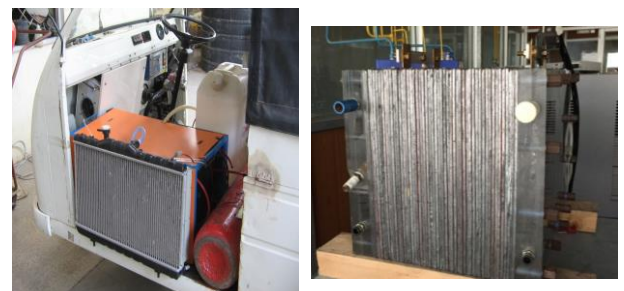
PEMFC stack with closed loop cooling and control system
